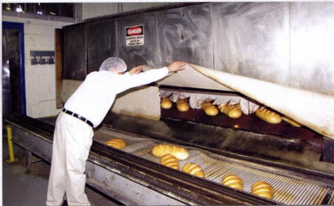
John Anthony Orlando shows off hearth baked Italian breads coming out of a 100-foot tunnel oven.
